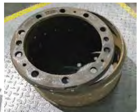
Failed aftermarket Scania drum ref; DVSA investigation Jan 20
