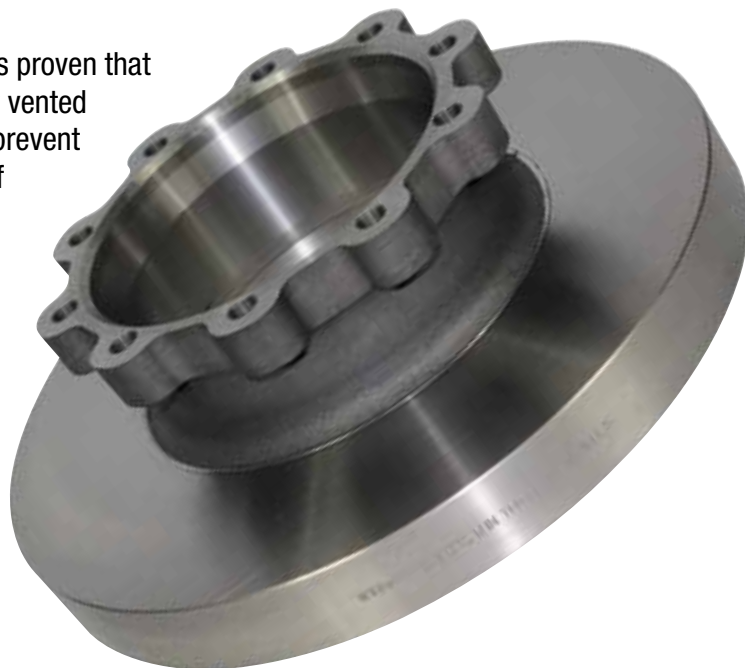
SOLID BRAKE DISC AFTER 15 BRAKE CYCLES Minimal heat crazing but no cracks
