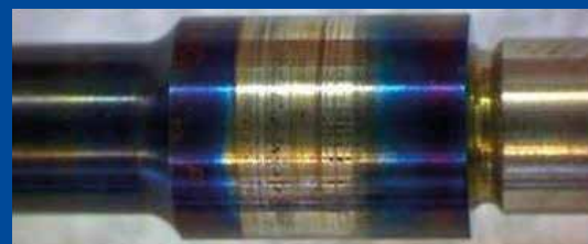
Evidence of overheating, caused by oil starvation
