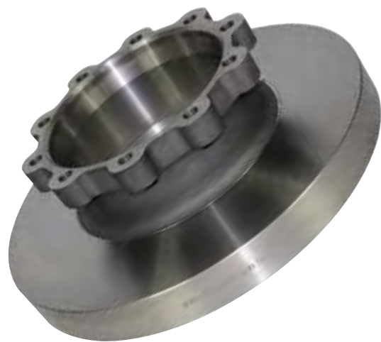
SOLID BRAKE DISC AFTER 15 BRAKE CYCLES
