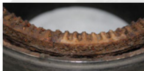
Decayed cast ABS teeth on an aftermarket disc:
