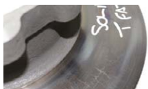
Close up of the solid disc front face after the ECE R90 comparison test
